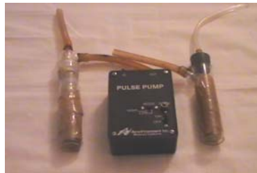
Fig 2. EBC collecting tube system and the pulse pump used for de-aeration of EBC samples.
